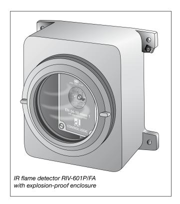
Normally the detector is installed vertically, centred on the area to be covered, so as the 90° cone field of view can be fully used. The ideal height is 0.7 the side of the square area.
